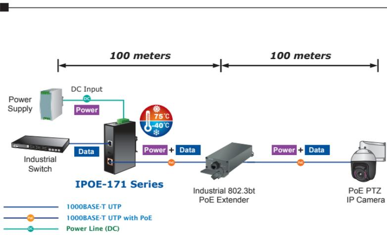
**Figure 16:** Connected Architecture of IPOE-171-60W and IPOE-E172
