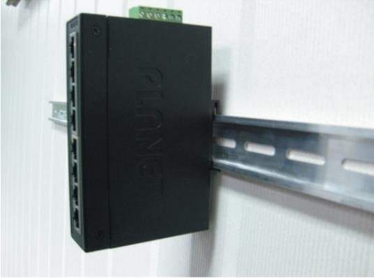
**Figure 11:** DIN-rail mount industrial device
