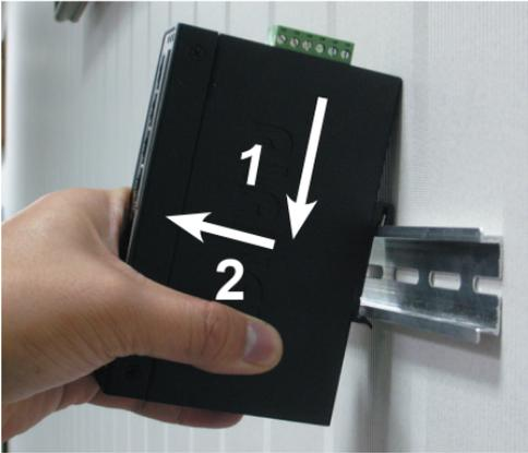
**Figure 12:** Removing industrial device from DIN rail
