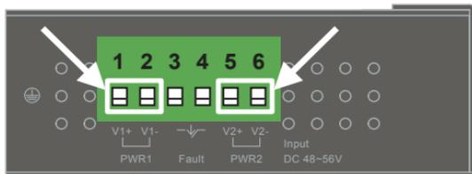
**Figure 6:** Power input pins.
