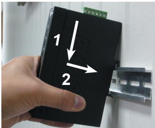
**Figure 10:** Mounting industrial device on DIN rail.
