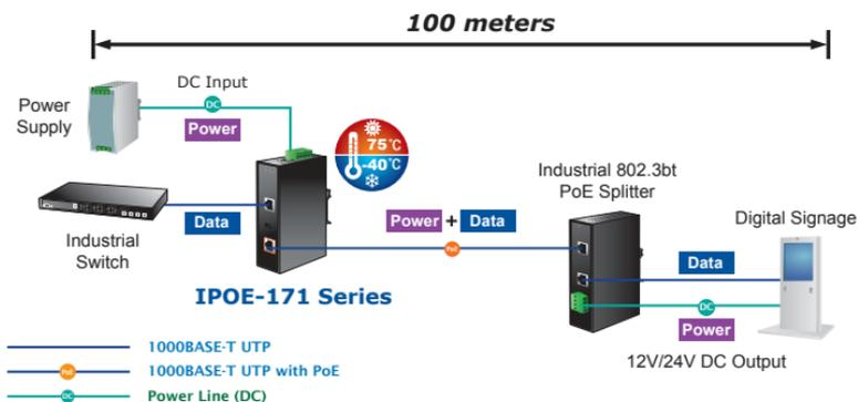
**Figure 15:** Connected Architecture of IPOE-171-60W and IPOE-171S
