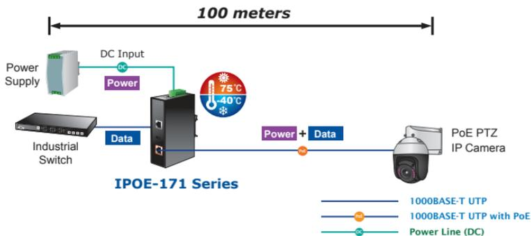
**Figure 14:** Connecting architecture with IEEE 802.3af/at/bt device
