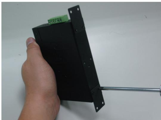
**Figure 13:** Attach brackets to the industrial device.
