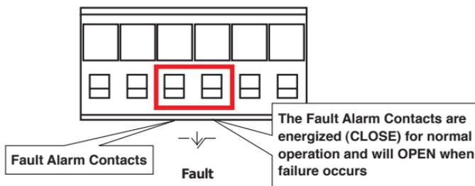
**Figure 9:** Fault Alarm Contact
